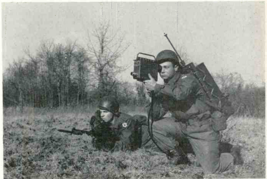
Shown in action is the new 55-lb. remote telecasting unit developed for the Army by Signal Corps Engineering Labs. Completely self-contained, the unit will transmit up to 1½ mi. Power is supplied by rechargeable 5-cell silver zinc batteries. Camera weighs 8 lbs., and includes 4 lenses, including wide angle and telephoto. Soldier at left is providing audio report over handle-talkie phone.
