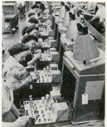
Assembly line at Bendix-Pacific looks like this as they swing into production on 57 new Bendix MR-3 Marine Radars ordered by U. S. Coast Guard for the service's patrol and rescue vessels
