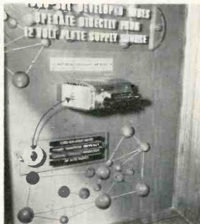
New tubes using 12 v. plate supply were introduced by Tung-Sol for auto radio production
