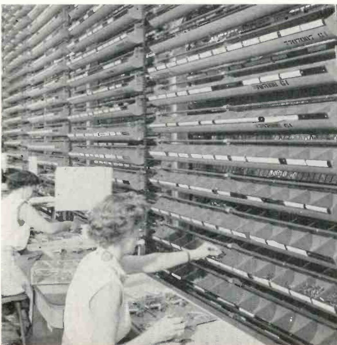
"Ferris wheel" arrangement of parts bins which move up or down by flip of a switch is used to speed assembly of military units at G-E's plant in Utica, N. Y. System was developed for specific needs of job-lot military electronics assembly work. "Ferris wheel," with 3,000 bins, occupies 150 sq. ft. of floor space
