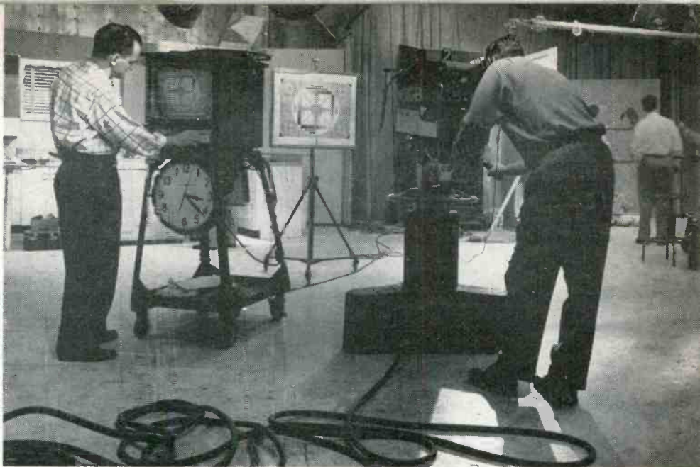
Fig. 5: Checking the gray scale with standard RETMA chart and normal lighting
