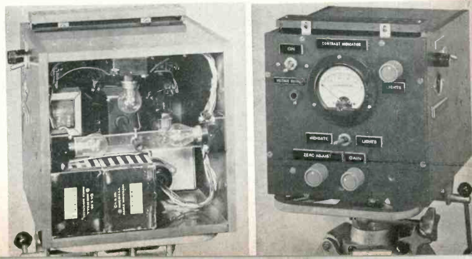
Figs. 2 & 3: Rear and front views of instrument. Contrast is read in percent change of indication
