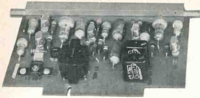
Fig. 1: Transistorized, printed circuit summing amplifier
