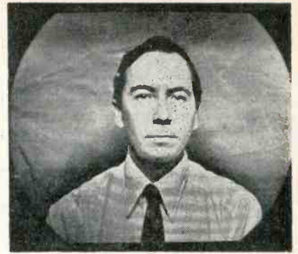
Fig. 8: Key to correct camera operation is seen in shadow above object's shoulders
