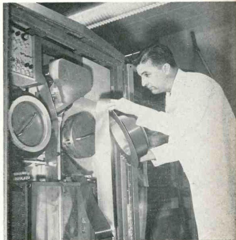
Single 2,700-ft. spool of magnetic tape shown being threaded into one of the 100 file units in the new "Datamatic 1000" computer by engineer Bob Wilkins, can store as much data on its 31 channels as can be found on a half-million punched cards.
