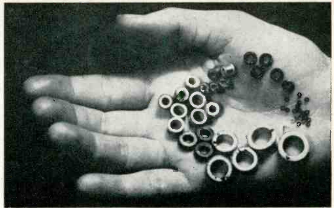
Fig. 1: Bistable ferromagnetic elements exist in 2 basic forms—microthin metallic tape and molded ferrites
