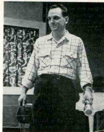
Fig. 2: Never carry tube face down
